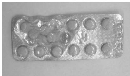
Fig. 1 Distension of the packaging material and release of tablets from PVC blisters
